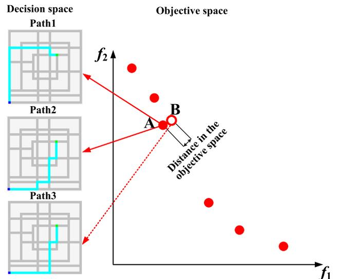
Fig. 3. Illustration of decision space and objective space of a dual-objective MMSPP. Due to the negligible distance between point B and point A, point B will be eliminated in the objective space, so path3 cannot become path2 by simply mutating.
