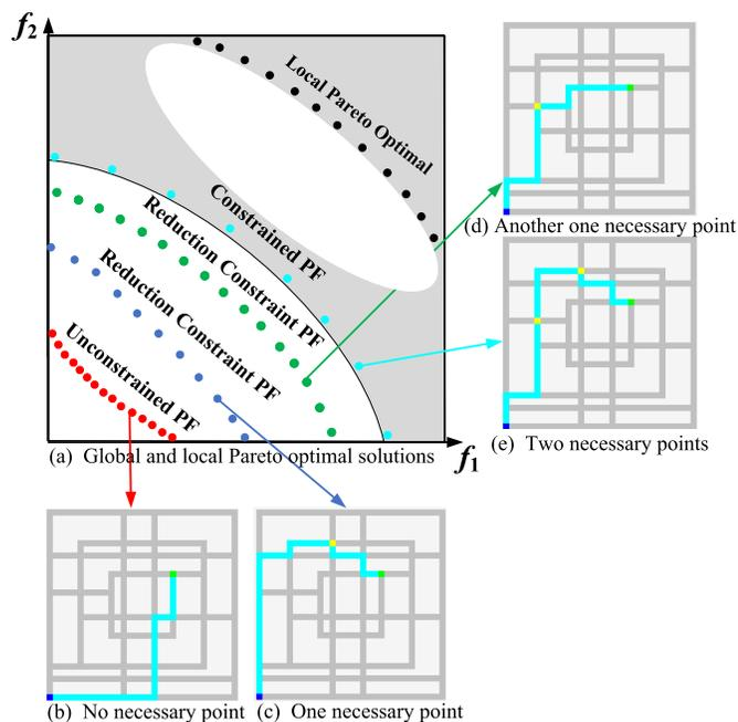
Fig. 2. Illustration of a dual-objective MMSPP with two necessary points. (a) The objective space of the MMSPP with a dual-objective and two necessary points. (b)-(e) The corresponding solutions in the objective space.
